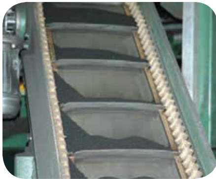
FRG - 3 Chemical powder conveying
